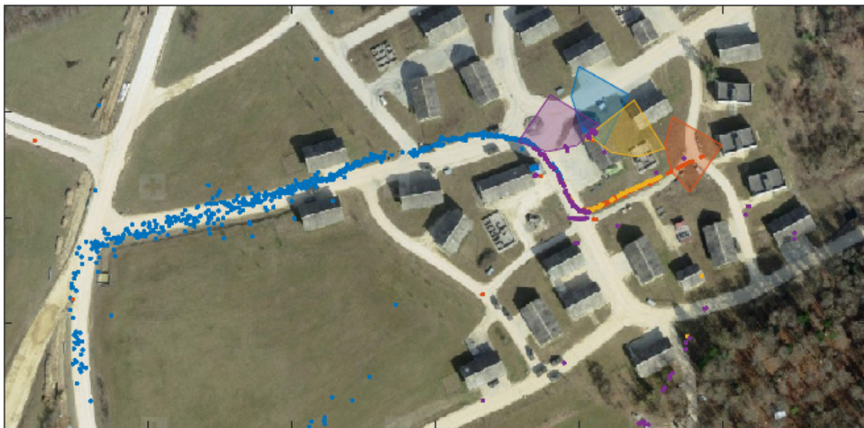
Figure 7: A fictitious UAV attack from the west to the target building (red sensor). The target enters the scene from the west and is first detected by the blue sensor node, followed by the magenta, the yellow and the red sensor node (coloured dots). The sensor positions and their field of view are shown by coloured sectors
